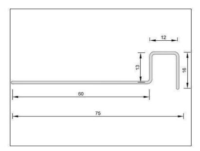
j) Only original JK manufactured "J" bite-bars of thickness 0.8mm to 1.2mm shall be used JK C 43 chassis.
